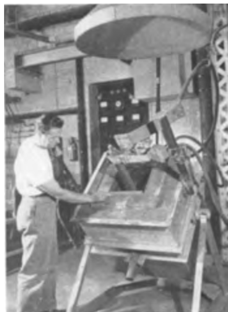
FIG. 6. Deep-shaft, single-phase electric furnace designed and constructed by the Bureau of Mines, used in studies on production of ferromanganese from domestic Mn ores.
