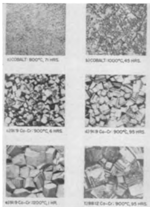
FIG. 5 (a-f). Photomicrographs of the outer surface of the scale formed on cobalt and Co-Cr alloys. Unetched and unpolished. 300\times before reduction for publication.
