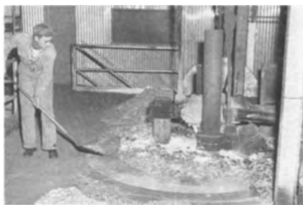
FIG. 3. Production of low-carbon ferrochrome silicon in ESB furnace.
