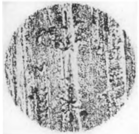
FIG. 8. Surface of as-machined vent plug (unetched—1500 X).
