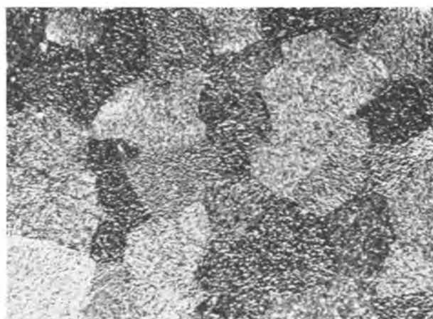
FIG. 4. Annealed chromium containing 0.022 wt % nitrogen, unetched. \times 22 .
