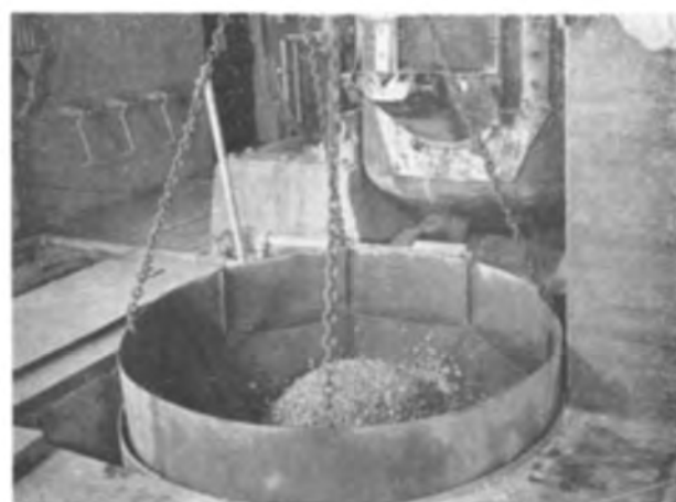
FIG. 4. Removing Co granules from quench tank
