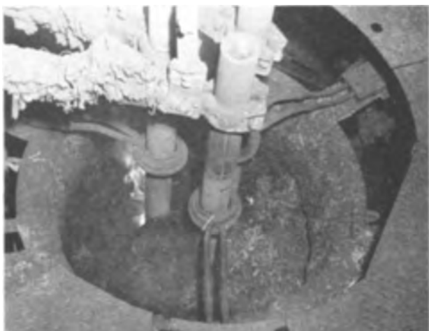
FIG. 2. Smelting nickeliferous Philippine laterite with bagasse in ESA furnace.
