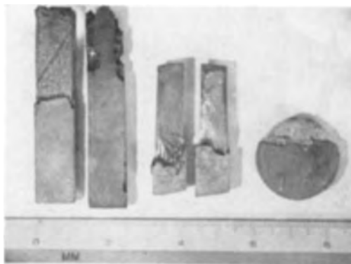
FIG. 5. The uncoated parts of iron, copper, and nickel samples are severely corroded by nitric acid.
