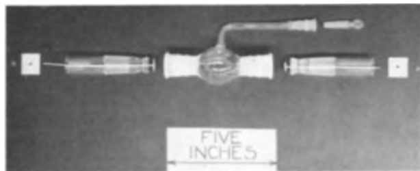
FIG. 1. Glass cell and copper electrodes used in this work to grow copper filaments electrolytically.
