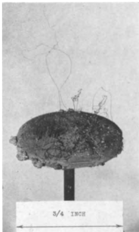
FIG. 3. Copper filaments grown with cetyl trimethyl ammonium bromide at 100 mg/l.
