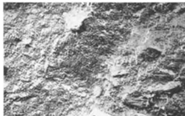
PLATE II. Chemically etched rolled copper anode in sulfate bath. 3000X.
