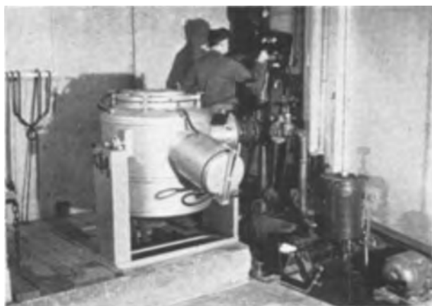
FIG. 7. With this vacuum melting induction furnace installation, 60-lb heats can be melted and cast at pressures below 10 \mu . Mn-Cu alloys are degassed at these low pressures and then melted and cast under a positive pressure of He to minimize Mn vaporization.
