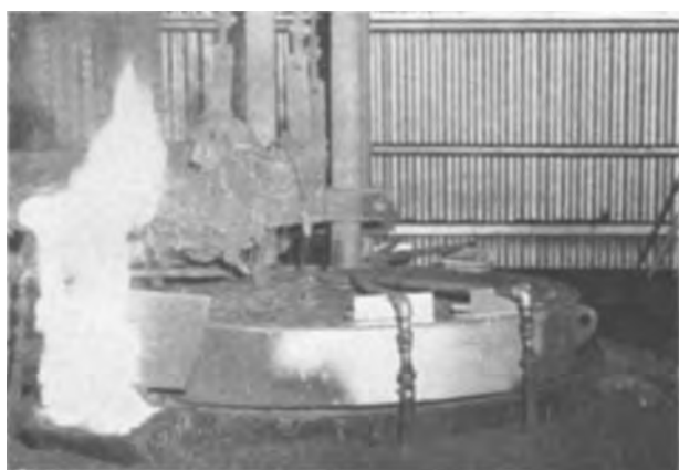
FIG. 1. Smelting siliceous Ni ore in roofed ESA furnace
