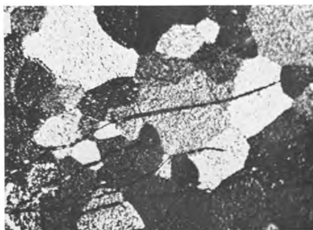
FIG. 5. Annealed chromium containing 0.022 wt % nitrogen made the cathode in an H_2SO_4 solution. Transcrystalline cracks developed. \times 22 .
