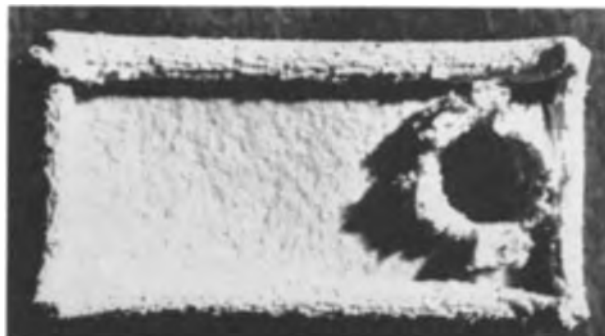
FIG. 3. Hot sheared tungsten sheet oxidized in excess of 850°C. Hot sheared; oxidized 25 min, 1000°C, 100 psia.
