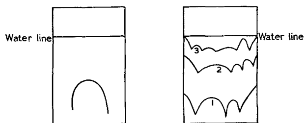
FIG. 13. Arch-shaped extensions of corrosion from a single point ( left ); successive positions of membranes ( right ).
