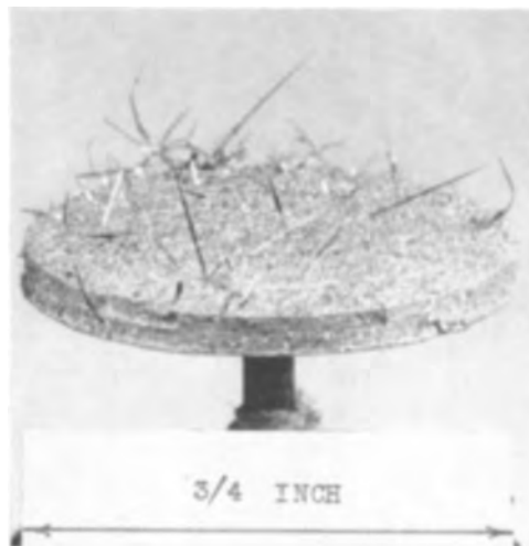
FIG. 2. Copper filaments grown with chloride at 10 mg/l using a current of 0.07 amp/dm 2 .
